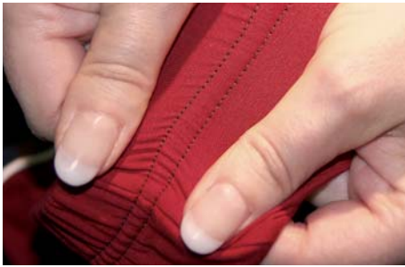
CHECKING SEAMS: SLIGHT PULLING AND SHEARING MOVEMENTS MAKE MATERIAL DAMAGE VISIBLE (FIG. 2)
